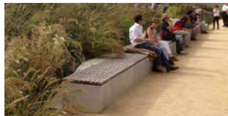
1 Furniture Type 1: Granite base with timber top. Wood Top System by Streetlife Finish: FSC timber Size: 500mm width, 480mm height.
