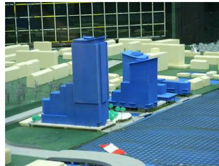
Photographs of BMT wind tunnel model from an earlier test day
